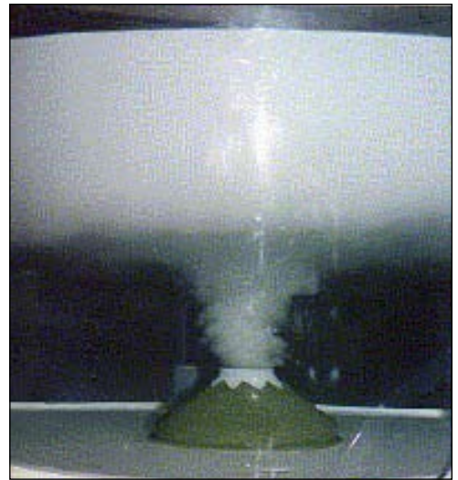
Figure 4: Result of injecting air into the suction of the Shearforce rotor
